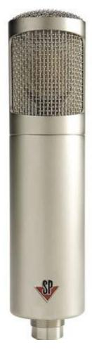
is a large diaphragm, fixed-cardioid condenser microphone employing a 1.06" (27mm) capsule, high quality, low noise amplifier and balanced, transformerless output circuitry. It features switchable -10dB or -20dB pad and 6dB@75Hz or 150Hz high pass filter for added control in various recording applications and a clear, full response expected from a large capsule microphone design.
